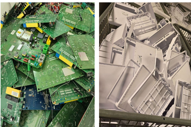
Image: Sorted PCBs ready for upcycling and sorted plastic housing from Icoteria routers ready for recycling.
